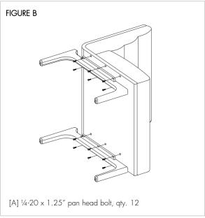
Note: Upon completion of Step 2, return the unit to upright position by lifting unit. Do not tilt or lean unit to upright position.
